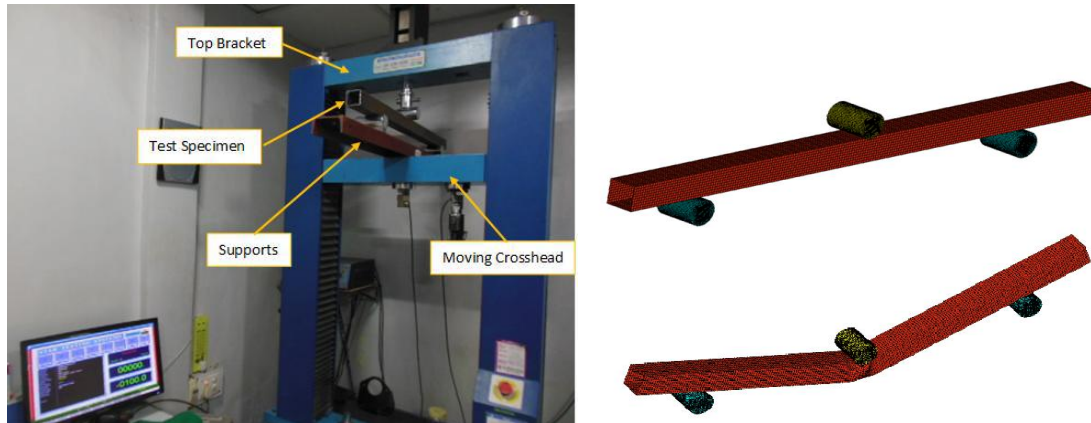
Fig.5 Three point bending test- experimental and Ls-dyna simulation
